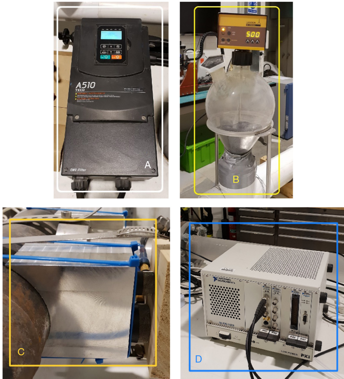
Figure 6: The flow loop facility components (A) Variable speed drive (VSD), (B) Hopper (sand injector device), (C) Ultrasonic sensor and metallic base, and (D) Data acquisition system.
