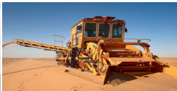
Fig. 2. SKM500 sand truck in Saudi Arabia (photo: Plasser & Theurer)
