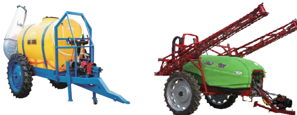
Fig. 3. Side blast sprayers: OVG-2006B and “Master” with drop-down consoles
