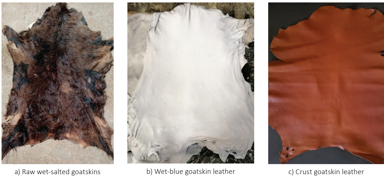
Figure 5. Enzymatically processed goatskin from the raw stage (a), through wet-blue (b) to crust stage (c)
