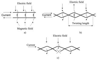
Figure 2 An electromagnetic field radiation by: a) flat cables; b) twisted cables; c) unbalanced cables
