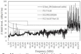
Figure 9 Comparison of the measured E-field radiation with proposed limits
