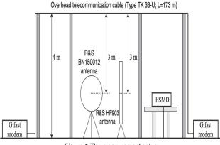
Figure 5 The measurement setup
