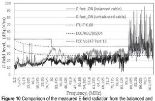
Figure 10 Comparison of the measured E-field radiation from the balanced and the unbalanced cable with proposed limits
