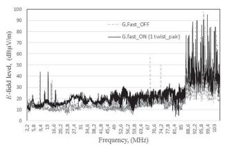
Figure 7 Measured E-field level in the frequency range from 2,2 MHz to 106,0 MHz
