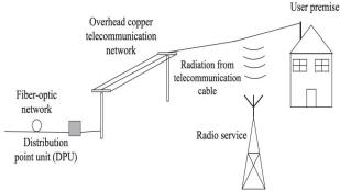
Figure 3 Radiation from telecommunication cable
