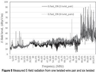
wire a measured E-field radiation from one twisted-wire pair and six twist wire pairs
