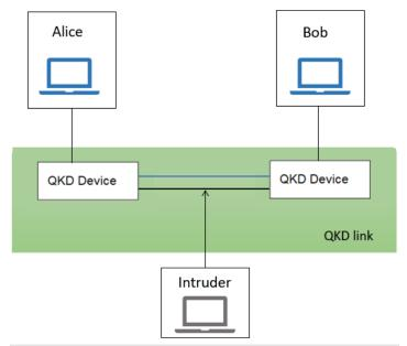
Figure 4. The intruder cannot break into the quantum channel (Source: Quantum-Safe Security Working Group)
