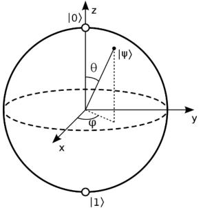
Figure 1. Representation of qubit states on a Bloch sphere (Source: Bloch, 1946)
