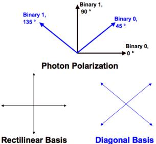
Figure 3. As seen on the Bloch sphere, each bit is encrypted with a rectilinear or diagonal basis, randomly chosen. (Source: Shukla and Patel, 2018)
