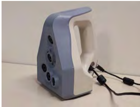
Figure 1. Handheld optical 3D scanner: Artec Spider, Artec 3D, Luxembourg.
