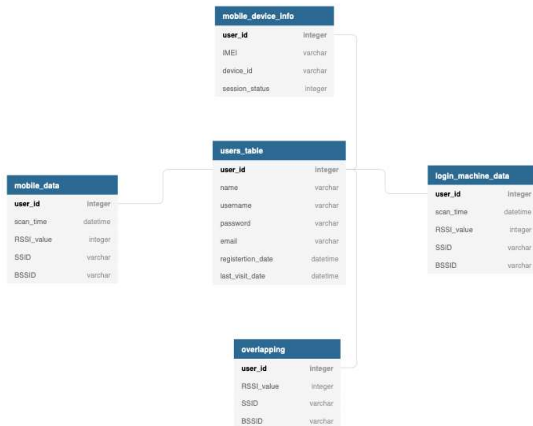
Figure 3-3: A simplified Entity Relationship (ER) diagram of the relational database used for the proposed system.
