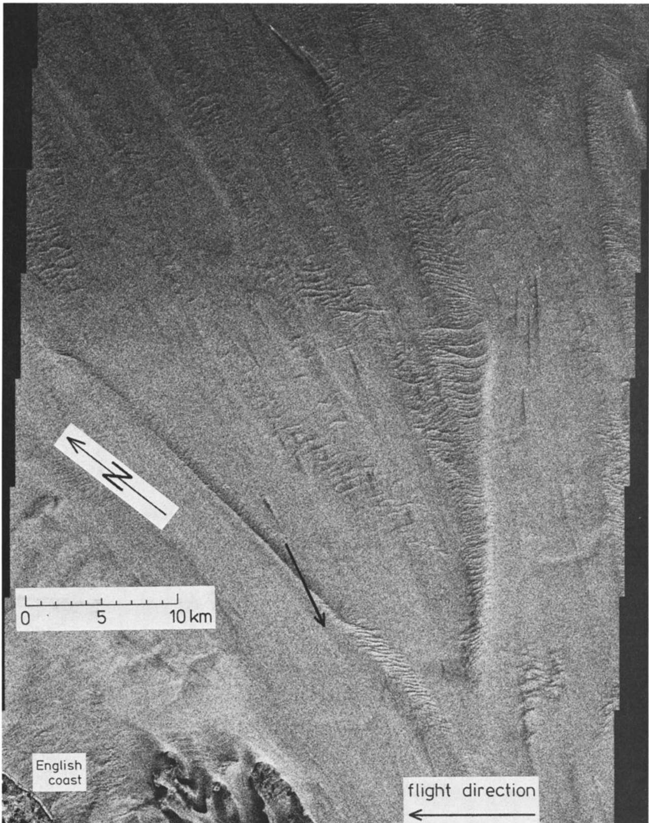
Fig. 5a. Digitally processed Seasat SAR image of the Southern Bight of the North Sea from orbit 762 (August 19, 1978, 0646 UT) with frame center at 51^{\circ}19'26''\text{N} , 1^{\circ}52'51''\text{E} . The land area in the bottom left-hand corner is the English coast near Ramsgate. The V-shaped feature in the center is the sandbanks South Falls and Sandettie.
