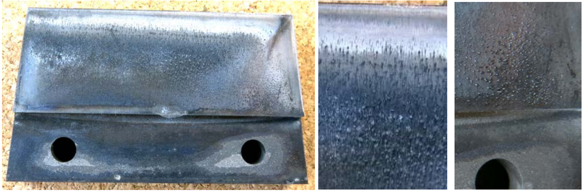
Figure 3. Tile 1e as seen visually. General view, surface close to the entrance to the gap, and surface close to the step near the SS holder.
