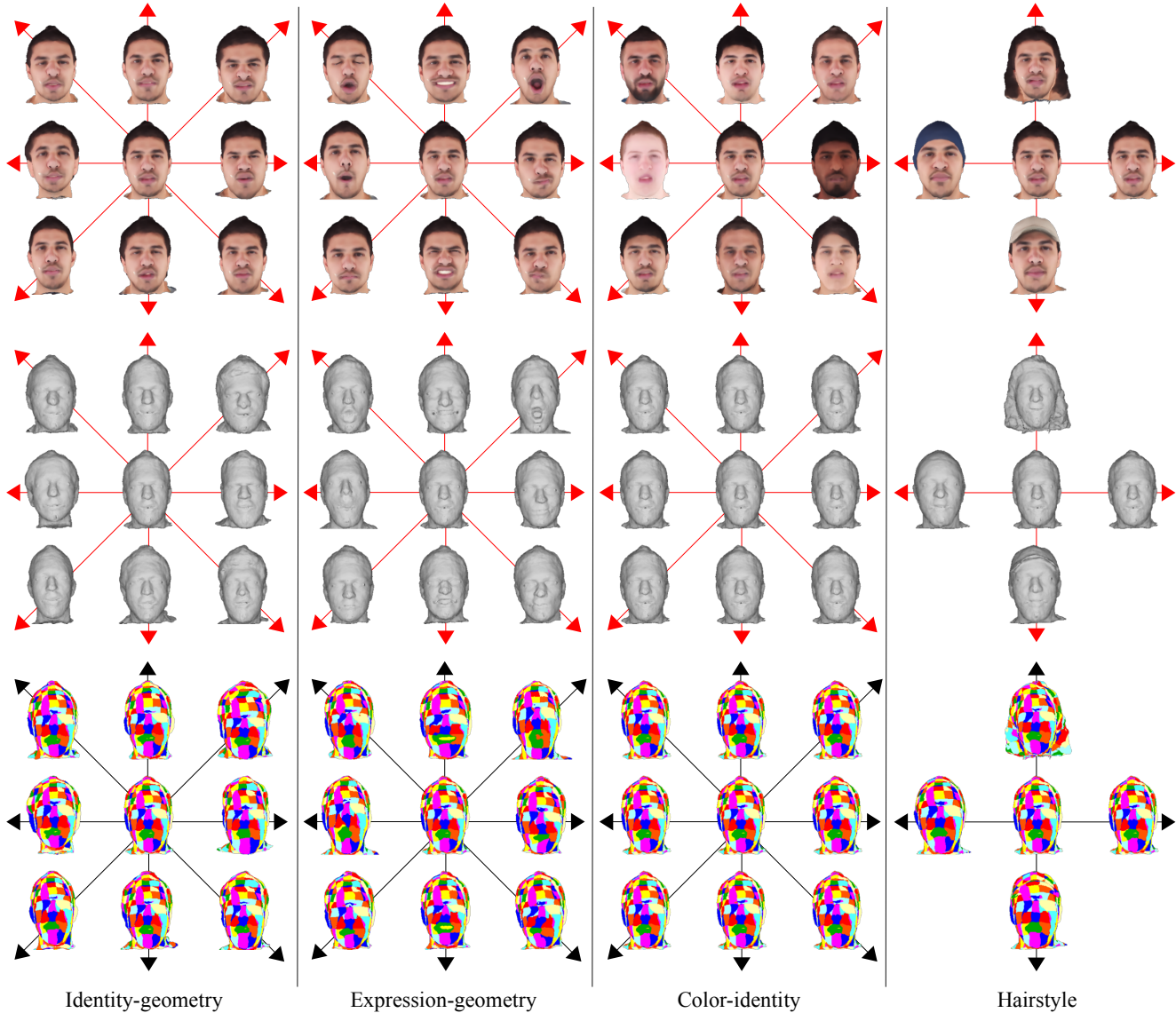
Figure 10. Principal components of different spaces i3DMM models. We show color renders at the top, geometry renders in the middle, and correspondences at the bottom.
