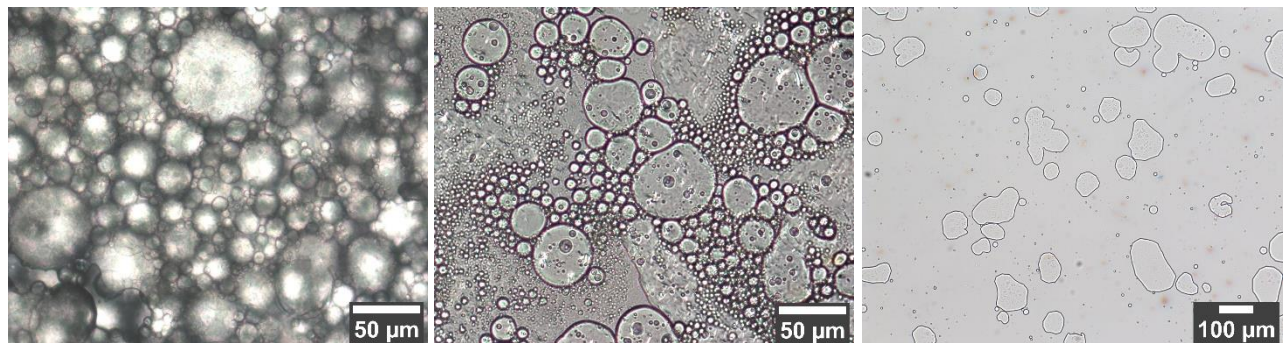
Figure 37: Comparison between emulsion prepared with SM, purchased at different times. Left: Emulsion prepared with SM purchased for pre-experiments, middle: Emulsion prepared with SM purchased for experiments, magnification 40x left: Diluted emulsion for experiments, magnification 10x.
