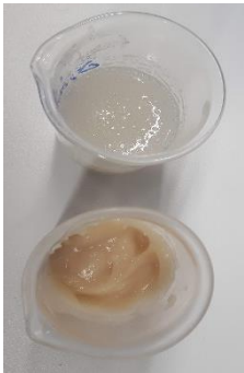
Figure 26: Soy protein dispersions with different soy protein content. Upper: 1 wt% SP, Lower: 10 wt% SP
