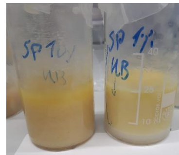
Figure 25: Phase separation after 30 min because of lacking mechanical energy. Left: CB emulsion prepared with 10 wt% SP; Right: CB emulsion prepared with 1 wt% SP.
