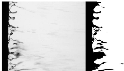
FIGURE 40. Original (left) and segmented (right) image using Otsu's method.
