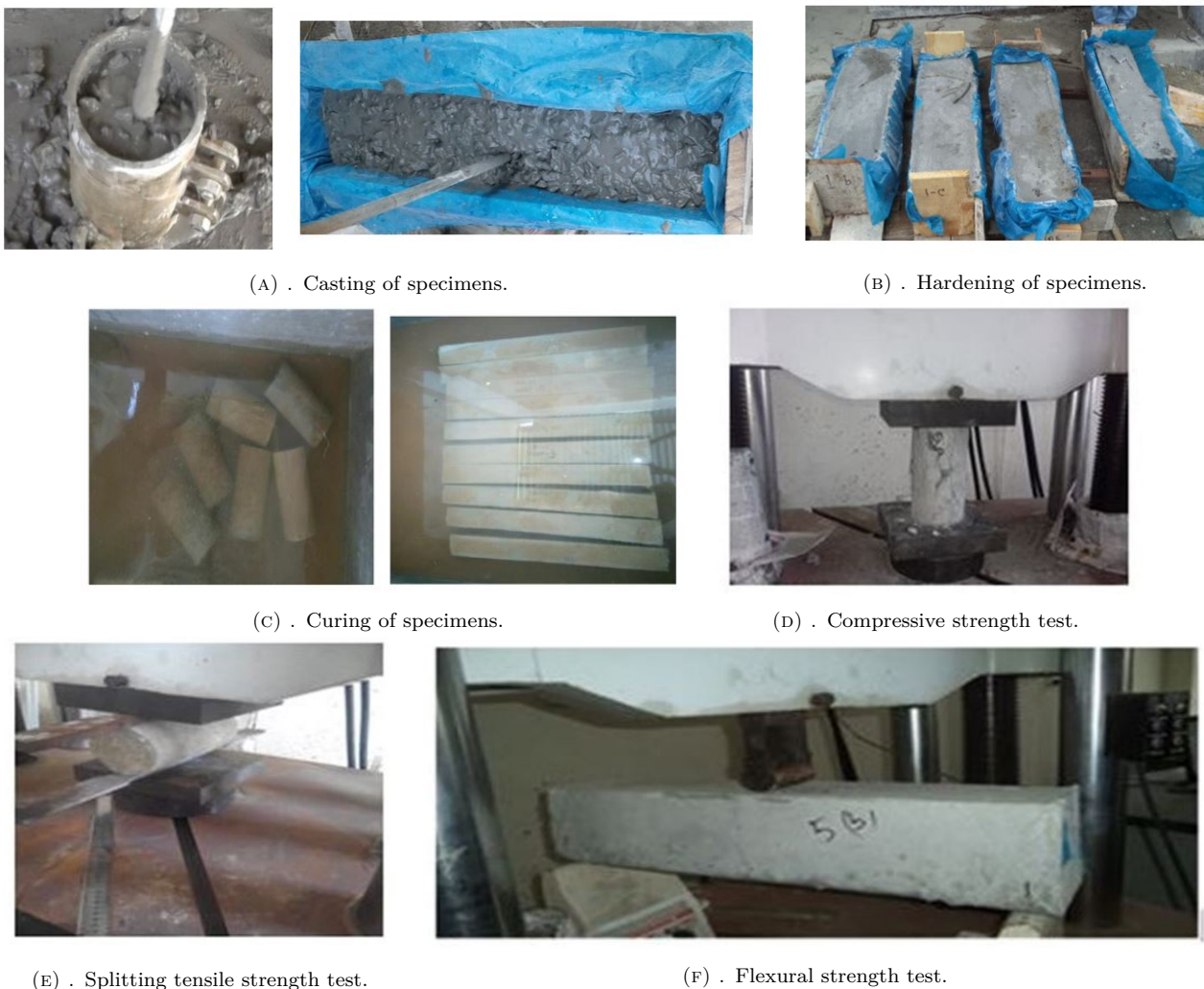
FIGURE 2. Specimen preparation and test setup.
