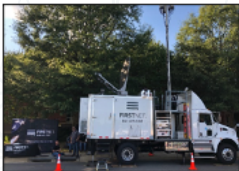
Figure 3: This AT&T SATCOLT is one of the tools that would have served as contingency communications infrastructure for JV 3.0 pre-COVID-19
