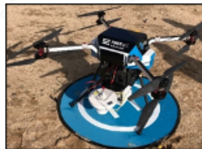
Figure 4: This AT&T cell on wings, also called a "flying COW," would have been one of the FirstNet-enabled devices provided during the JV 3.0 LFX.
