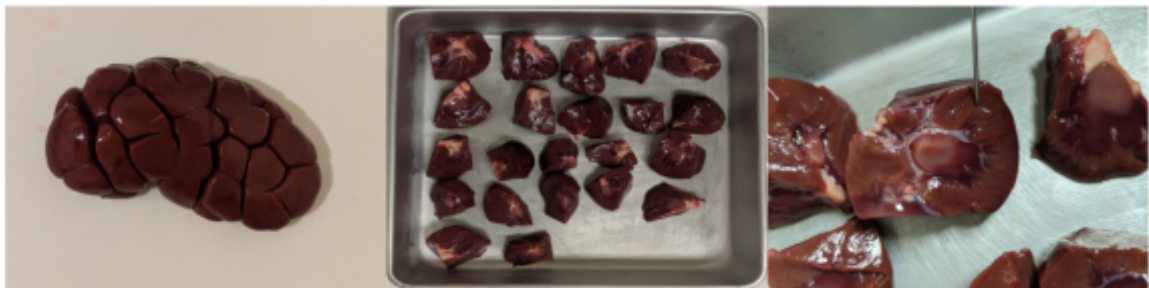
Figure 2.6: Preparation of the bovine kidney samples. The kidney was sectioned into 22 pieces and placed on an aluminium tray. The needle was inserted into the same location across the other samples. The other ex-vivo tissue samples received similar preparation.
