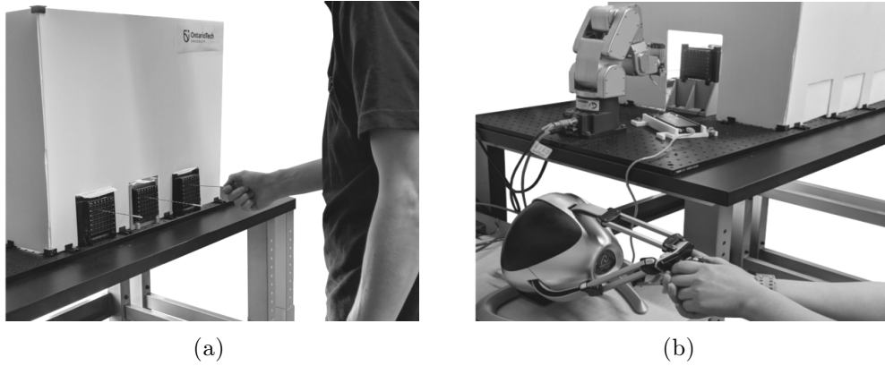
Figure 5.10: The two stages of the user trials. (a) The test participant would first insert the needle by hand to determine the depth of the cancer layer in the unique phantoms. (b) The participant would then determine the depths using haptic feedback in the teleoperated scenario.
