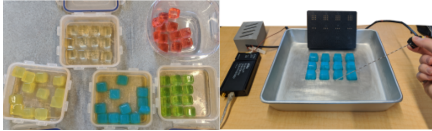
Figure 2.5: The gelatin and agar samples were prepared using their corresponding recipes. Pictured here are Gelatin (Original), Gelatin (Red), Gelatin (Green), Agar (Blue), and Agar (Yellow 2).
