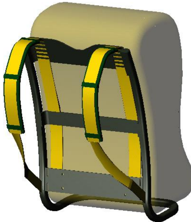
Figure 2.5 Schematic of the energy harvesting backpack with piezoelectric straps [32]
