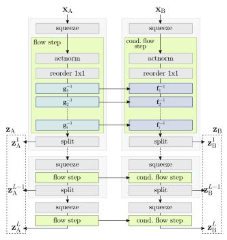
Figure 2: The C-Flow model consists of two parallel flow branches mutually interconnected with conditional coupling layers. This scheme allows sampling  $x_B$  conditioned on  $x_A$ . For a detailed description on functions in grey refer to [25].
