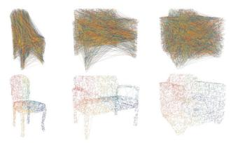
Figure 4: Sorting 3D point clouds. Point clouds corresponding to three different chairs. The colored line connects all points based on their ordering. **Top:** Unordered. **Bottom:** Applying the proposed sorting strategy. Note how the coloring is consistent across samples even for point clouds with different topology.
