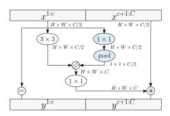
Figure 5: Approximating global features in point clouds. When dealing with point clouds (reordered and reshaped to a  $H \times W \times 3$  size and using c = C/2) we approximate, with operations in blue, global features in coupling layers while still being invertible.  $\circledast$  stands for affine transformation where the first C/2input channels are the scale and the other half the translation.
