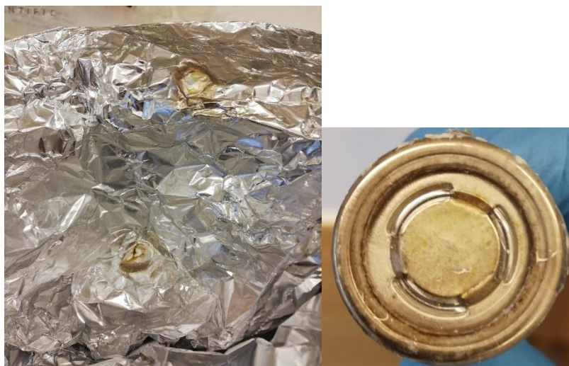
Figure 37: showing corrosion of (a) aluminum foil and (b) positive terminal
