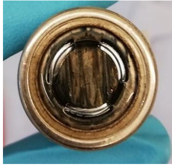
Figure 28: deposition onto the positive terminal in the \sim 45^{\circ}\text{C} solution
