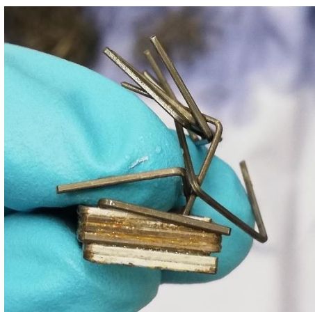
Figure 43: showing rusting of the staples post discharge in run 1
