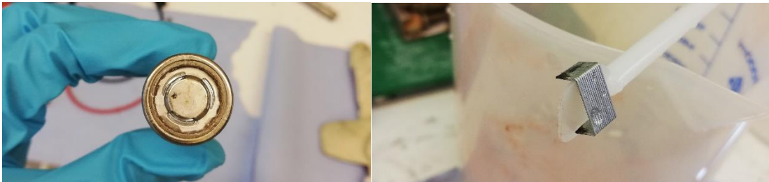
Figure 39: showing melting of the casing and staples as a result of short circuiting
