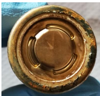
Figure 18: Corrosion of the cell casing in the 2 nd hour
