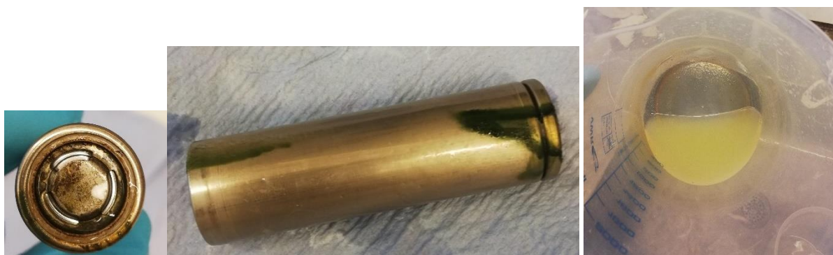
Figure 32: showing (a) corrosion of the positive terminal after 24hrs of 10wt% discharge (b) blue-green bacteria forming on the cell in the heated solution (c) yellow translucent solution formed at the end of the heated experiment
