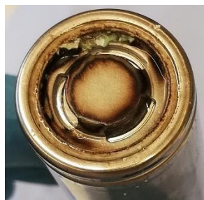
Figure 22: showing corrosion at welding points and blue-green crystal formed in \text{NaNO}_2 solution
