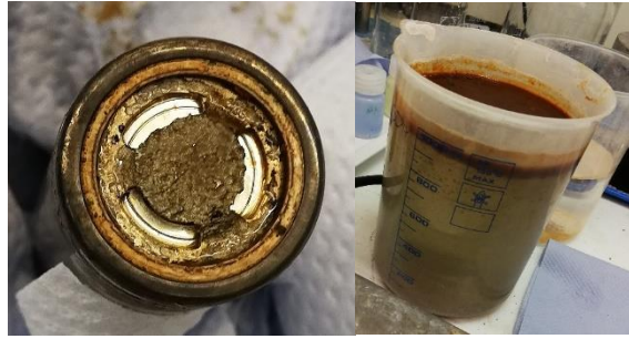
Figure 16: showing (a) corrosion of the casing after 6 hours, (b) orange-brown film at the surface of the solution after 6 hours
