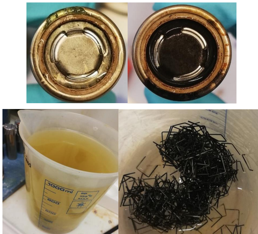
Figure 48: showing (from top left) (a) corrosion of the casing and formation of blue-green bacteria after one hour (b) blackening of the positive terminal after 24 hours of discharge, (c) yellow-brown solution post discharge, (d) blackening of the staples post discharge
