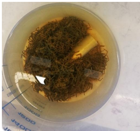
Figure 41: showing rusted staples after 24 hours in water
