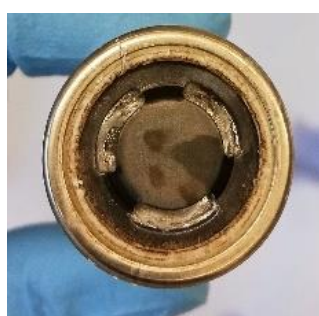
Figure 24: uniform corrosion of positive terminal
