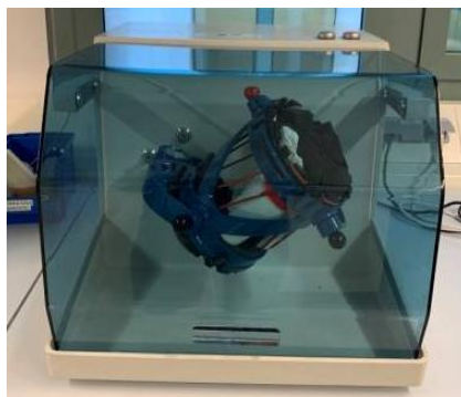
Figure 4.5: Image of Turbula ® machine used during this Master's project.
