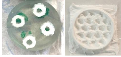
Figure 1.1: Electrolyte geometries from the Bachelor's project. Left: tubular geometry and right: hexagonal one.
