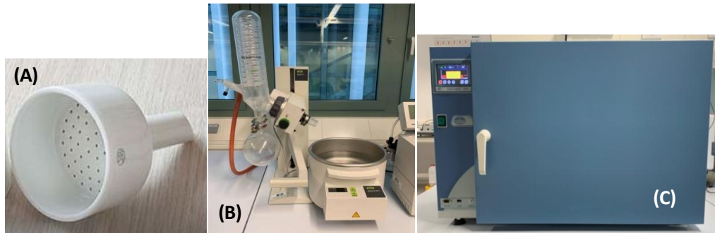
Figure 4.6: a) Büchner funnel to detach the alumina mill-balls from the mixture, b) steam rotavapor used to separate the ethanol from the ceramic powder and c) stove to dry the final mixture powder.
