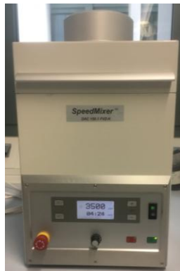
Figure 4.8: SpeedMixer, the machine used to mix the hydrogel and ceramic pastes.
