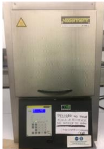
Figure 4.11: Furnace where the printed specimens were sintered.
