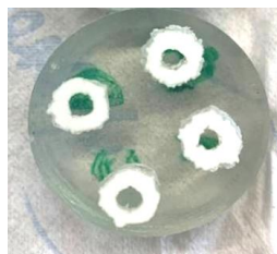
Figure 4.14: Zirconia samples embedded inside the resin to polish them.
