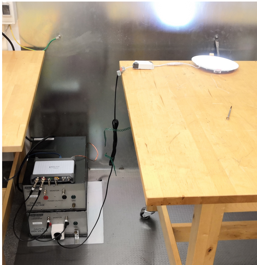
Figure 1: Close look at the GCEM's conducted emissions setup while a test is being performed. The EUT is connected to one of the LISNs inputs (bottom left) and their outputs are connected to the receiver. Note that the EUT is positioned at a predefined distance from both horizontal and vertical ground planes.
