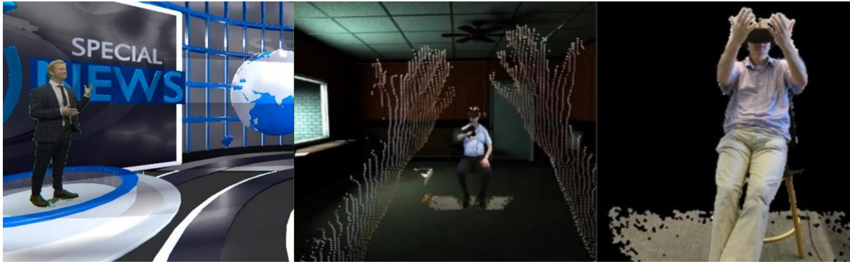
Figure 2. Scenes from VRTogether [4]. From left to right: recorded 2D video presenter using chroma inserted in a CGI scenario, point cloud self-representation and point cloud representation of the partner.
