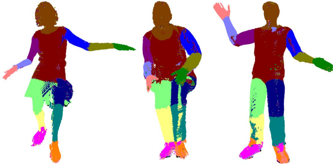
Figure 23. Point cloud resulting of the reconstruction using the 2D approach to remove the background
