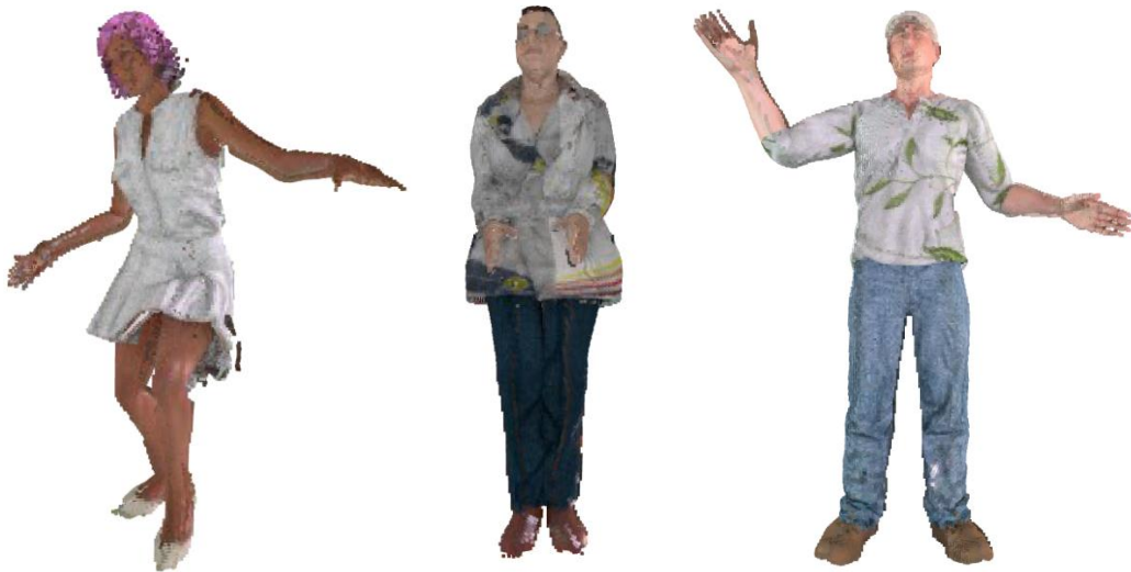
Figure 21. Resulting point clouds reconstructed after applying the correction to the depthmap.
