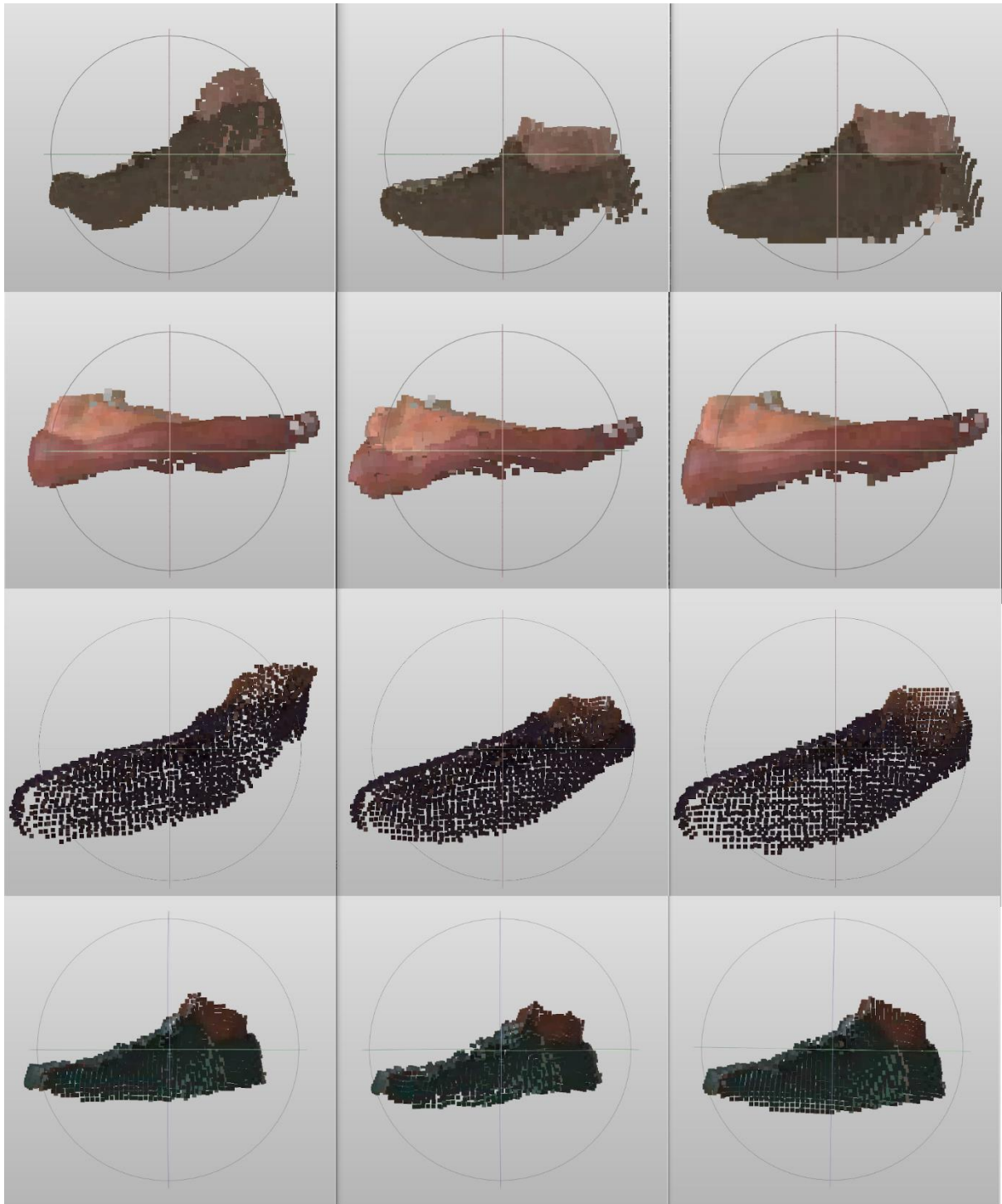
Figure 58. Visual comparison of the prediction of the foot using both models in Experiment 4. Left: using M_{fb} . Middle: using M_{feet} . Right: groundtruth
