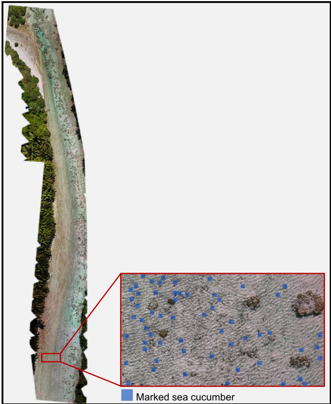
Figure 4. Photomosaic map of study region in Tetiaroa, French Polynesia generated by stitching 56 overlapping, geo-referenced images using the application Pix4DCapture. Inset highlights zoomed in portion of image with sea cucumbers manually marked using Visual Counter.
