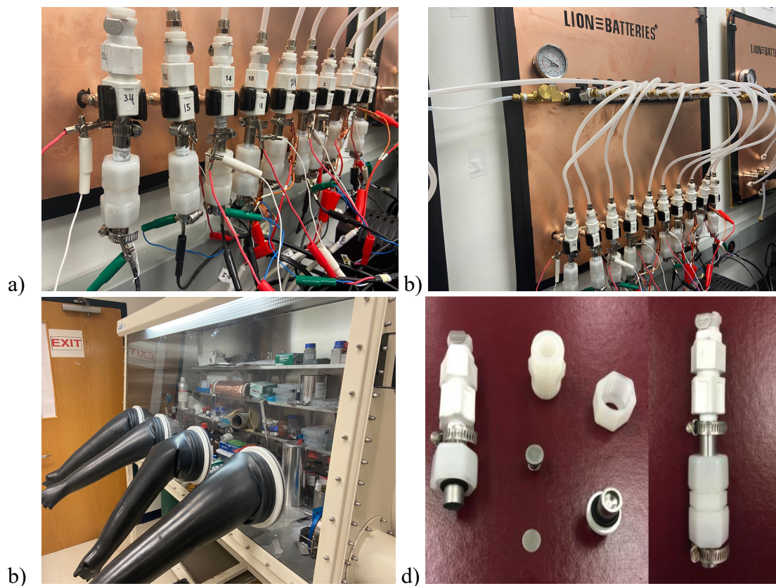
Figure 15. Pictures of a) Swagelok cell mounts, b) oxygen inlet tubes, c) Argon-filled Glove box, and d) disassembled cell (left) and assemble cell (right).
