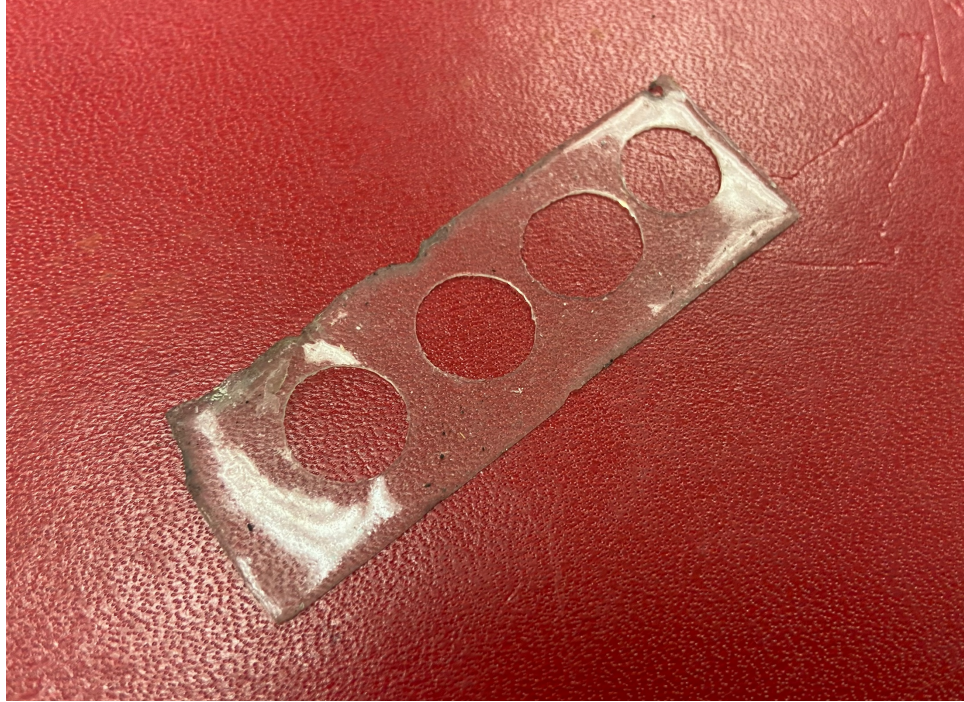
Figure 40. Illustration of a PDMS template used for GPE/cGPE disc polymerization.
