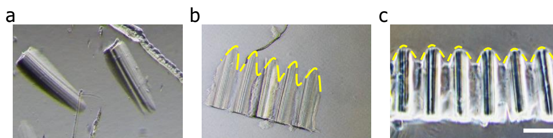
Figure 4.59. Images of the cross-sections of the microstructured hydrogels showing a single row of the villus-like structures. It can be easily appreciated material crosslinking between pillars, which increases when the energy dose applied increases (a) 4.9, (d) 5.9, and (e) 7.5 J·cm -2 . The borders of the pillars are marked in yellow. Scale bar: 500 μm.
