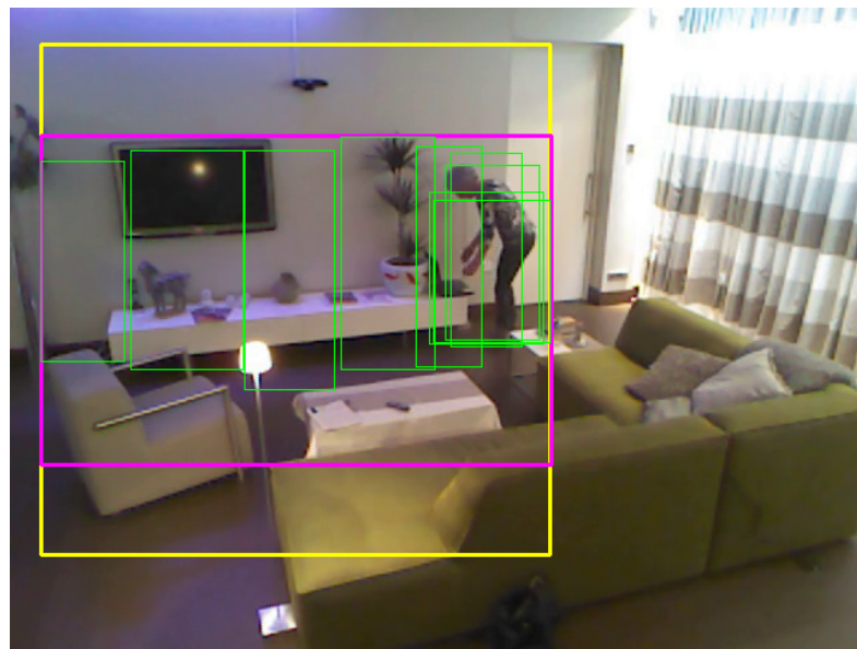
Figure 3. Frame from a 'Walk' sequence showing the full crop concept: a crop involving the full area where the activity takes place (bounding box in purple). The yellow bounding box shows the square area of the final image crop. Bounding boxes of each separate detection shown in green. For visibility, only one in every 10 detections (green bounding boxes) is shown.
