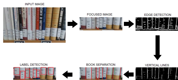
FIGURE 7. Our vision approach to separate book by book and extract each tag with the book code.
