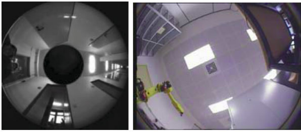
FIGURE 1. Difference between a catadioptric image (left) and a fisheye image (right).
