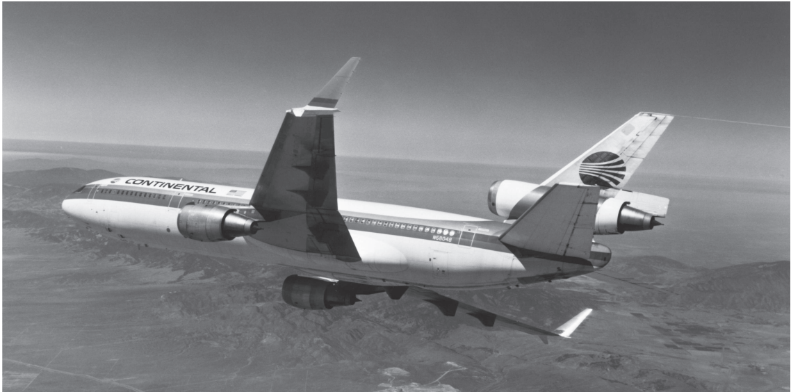
Fig. 1.8: Experimental McDonnell Douglas DC-10 commercial aircraft equipped with winglets performing a flight test.
