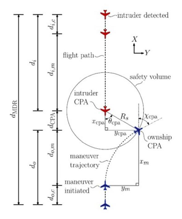
Figure 2.21: The Total Minimum Detection Range,  $d_{MDR}$ , Needed and a Representation of the CPA [119]
