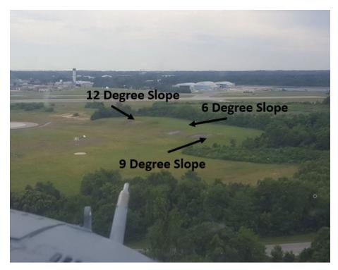
Figure 4.5: Pilots Perspective of Surveyed LZ Used for Slope Landing Evaluation Taken from a UH-1 at 200 ft AGL Over the Turf Training Area of NAS Patuxent River [140]
