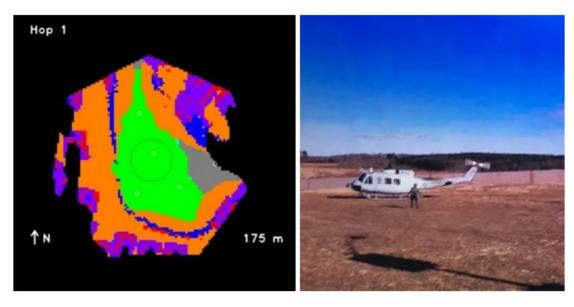
Figure 4.7: Two Images Relating to an Autonomous Landing in a Field During Flight 59F098 Left: TALOS Interpretation of the LZ [132] Right: Picture of the Test Vehicle Shortly After Completing an Autonomous Landing in the LZ Pictured on the Left [141]
