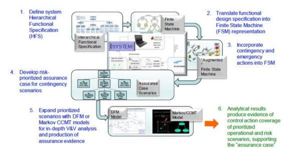
Figure 2.20: MBCS V&V Framework Process Flow and Elements [63]
