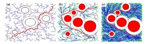
Figure 2.22: RRT and RRT\* Path Planning. Image (a) is an Example of RRT, Which has been Widely used for Path Planning of Autonomous Robotic Path Planning. Image(b) is a Midpoint of the RRT\* Algorithm Where it is Defining a More Optimal Path Through the Obstacles. Image (c) is the Final Product Where the RRT\* Algorithm has Defined the Optimal Path Around the Obstacles [122]
