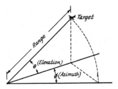
Figure 5.4: Graphical Depiction of the Three Possible Error Parameters of the Sensors Installed on the Bucket Fighter [179].
