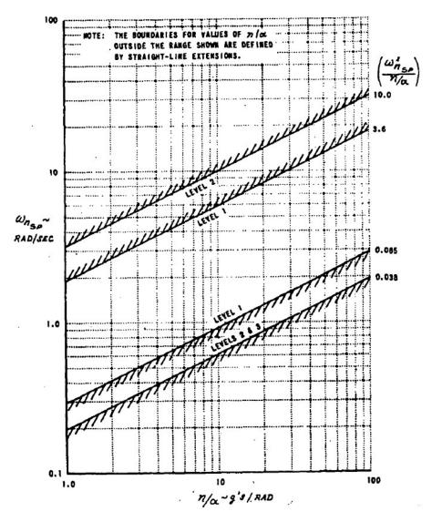
Figure 5.2: Relating Short Period Aircraft Dynamics to Aircraft Handling Qualities Levels During Nonterminal Flight Phases that are Normally Accomplished Using Gradual Maneuvers and Without Precision Tracking, From Mil-F-8785C [171]
