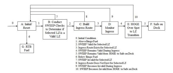
Figure 3.1: State Machine Specification Which Details the Decision Process for a Unmanned System to Make a Decision Currently Reserved for a Qualified Pilot
