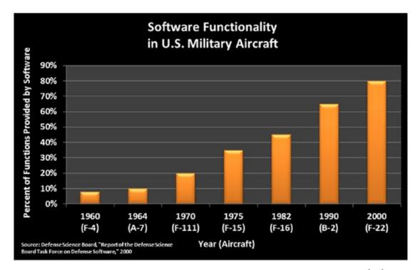
Figure 2.14: Increasing Aircraft Functionality Provided by Software [21]
