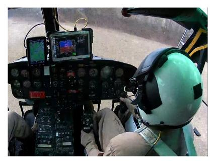
Figure 4.13: Image From the System Under Test During the 23 January 2018 Flight. At the Depicted Point During the Flight the Systems SA of the Environment Didn't Match Reality. The Autonomous Functionality would have Flown Through Some Trees and Caused a Mishap if the Safety Pilot Didn't Take Control of the Vehicle [132].
