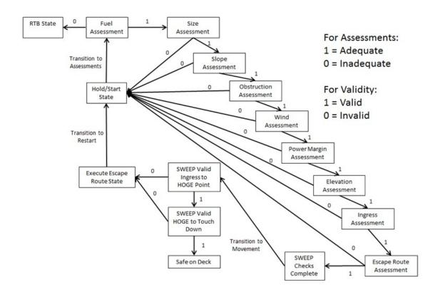
Figure 3.6: Protocol Which Meets the Requirements of the Specification Detailing the Decision Process for a Unmanned System to Make a Decision Currently Reserved for a Qualified Pilot
