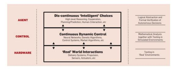
Figure 2.12: Typical Hybrid Autonomous System Architecture – with Suitable Analysis Techniques Noted in Reference [24]
