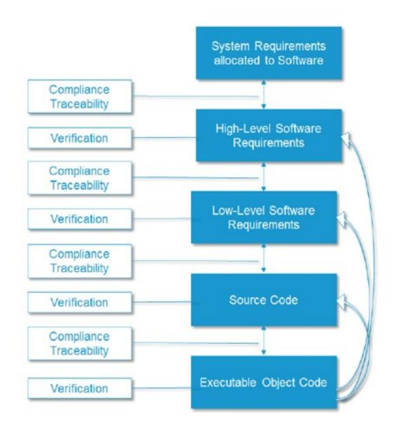
Figure 2.15: Important Development Phases According to DO-178C, Including the Necessary Verification Steps (Architecture Design and Verification have Been Omitted) [26]
