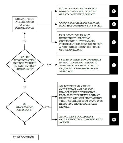
Figure 5.3: PALS/Pilot Quality Rating Scale, Allows Test Pilots to Objectively Gage their Confidence in the System Under Test. Developed for PALS Testing [2,86], and it has Been used for Evaluation of Autonomous Systems [136]
