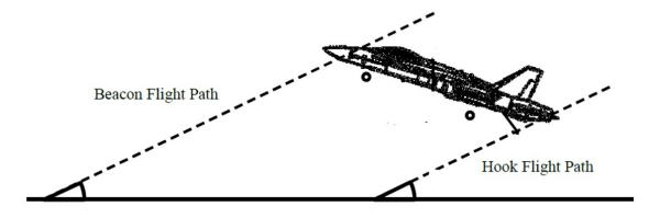
Figure 2.4: Graphical Depiction of the Difference Between the Beacon and Hook Flight Path on PALS Approach [86]
