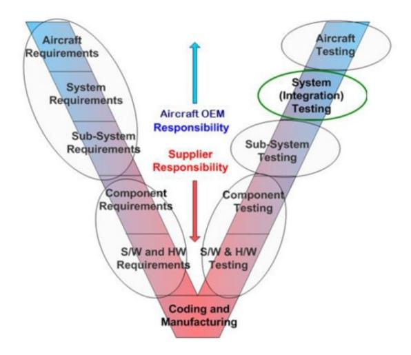
Figure 2.18: V-Cycle Stages for MBD-Based V&V [22]
