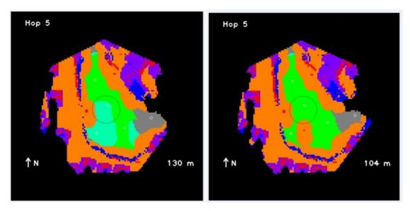
Figure 4.9: TALOS Interpretation of an LZ Before (Left Image) and After (Right Image) a Golf Cart if Driven Into it Testing the Wave Off Functionality on Flight 59F096 [132]
