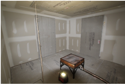
(c) Bedroom 1 Propane Burner and Thermocouple Tree
