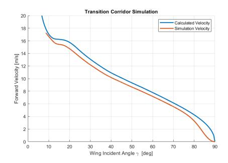
Figure 4.1: Comparison of calculated transition corridor and a simulated transition corridor.
