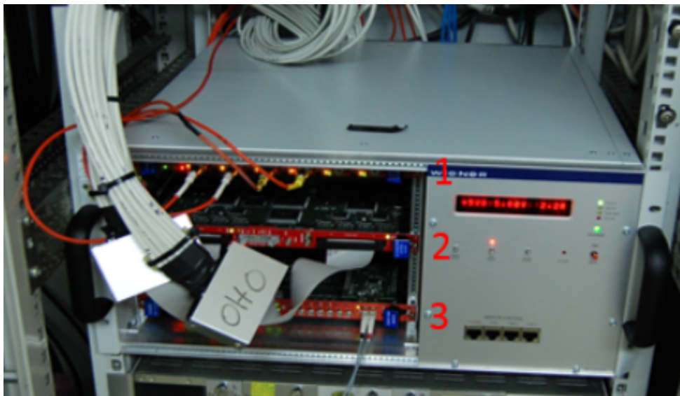
Figure 3.9: In this photograph we can see the card with high voltage for the PMT (1), the cables from the OB with digital signal connected to the CAEN counter card(2) and the communication cable of optical fiber from CAEN to labm-computer (3).
