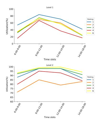
Figure 11: Percentage of average utilization of a) Level 1, and b) Level 2 chargers during each time slot in five parking lots
