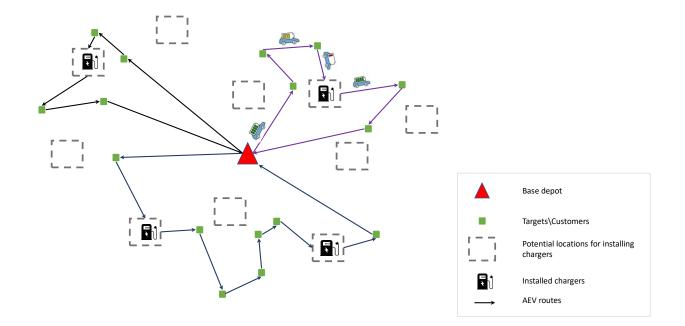
Figure 1: The relationship between the charging location decisions and routing strategies for autonomous electric vehicle's operation
