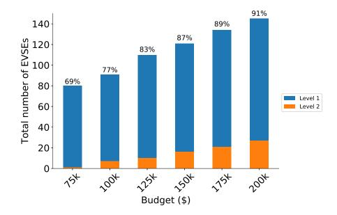
Figure 9: Number of installed level 1 and level 2 chargers for different budget amounts, labeled by accessibility percentages.
