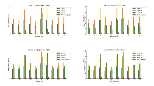
Figure 13: Aggregated EV drivers' utility of using different charger levels in different parking lots when the level 3 charging price is 9(\$/h), 6(\$/h), 4(\$/h) and 3(\$/h)
