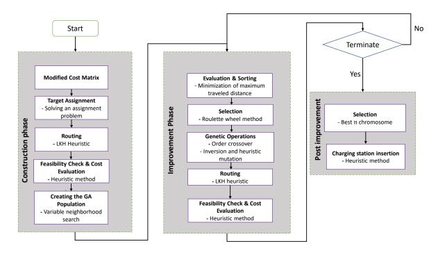
Figure 16: The flowchart of GAH including three main phase : construction, improvement and post improvement
