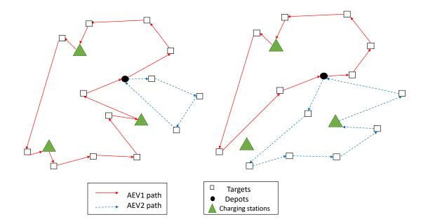
Figure 15: A feasible tour for two AEVs which visit all the targets while visiting some charging stations for recharging: AEVRP using min-sum (left) vs AEVRP using min-max (right).
