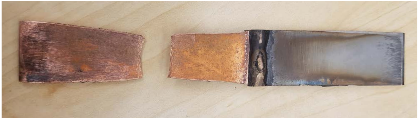
Figure 1: The Cu-SS weld is stronger than the copper base material.
