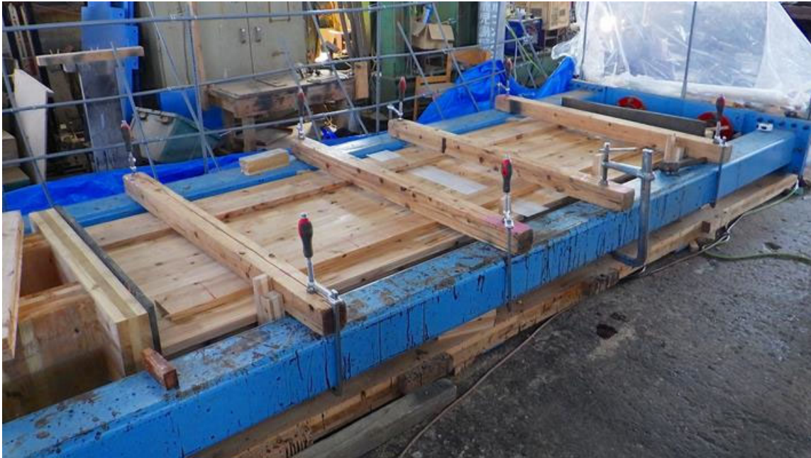
図 3 Fig.3 Situation of jointing a few test specimens in the prototype device
