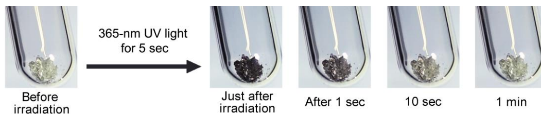
Figure 2. (a) Photographs of the photochromic reaction of the powder of 1% Cu-doped ZnS NCs upon UV light irradiation (365 nm, 500 mW cm -2 ).
