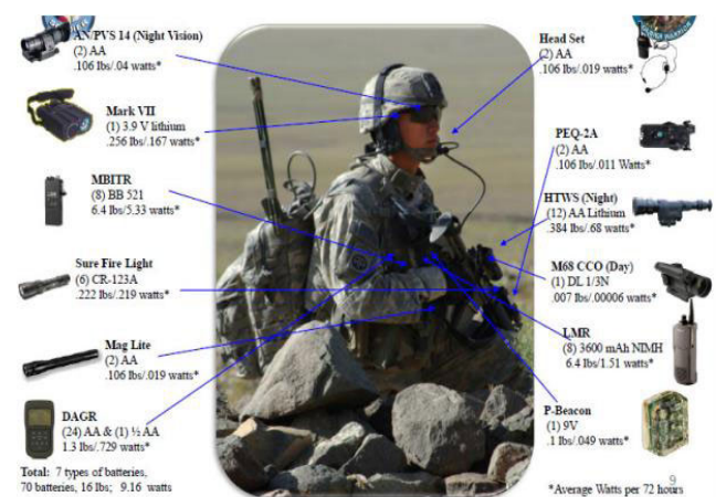
FIGURE 1. Devices and batteries used by a US soldier during an operation – carrying a total of 70 batteries weighing at 7kg [9].
