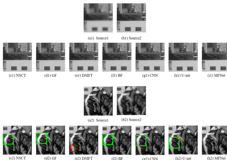
Figure 8. Magnified regions of the “Model Girl” source images and fused images obtained with different methods.
