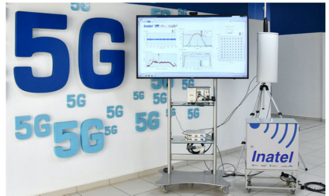
FIGURE 15. 5G-RANGE BS prototype implemented using National Instruments equipment.
