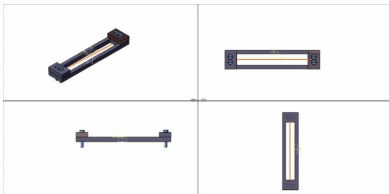
Figure 6: Design of the support for the copper microwire, which was designed to allow for the correct introduction of these wires into a liquid medium. One edge of the support has a copper contact, place where the power unit would be connected to.
