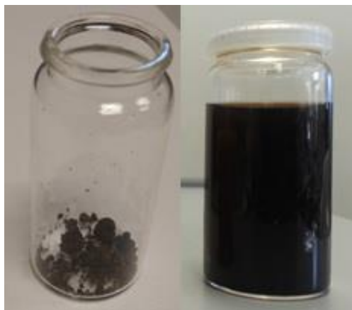
Figure 1: Left, Graphene oxide after lyophilization. It forms a powder which can then be dispersed in water (right), to form a graphene oxide aqueous dispersion. It is important to use ultrasonication as means for the correct dispersion of the graphene oxide, as otherwise powder deposits could be found in the liquid medium.
