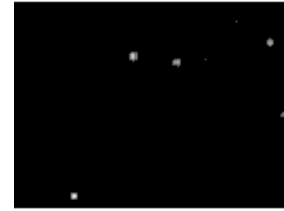
Fig. 11. Example of final preprocessed star tracker image.
