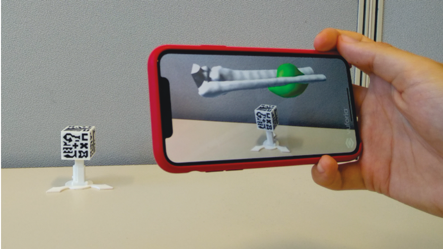
Figure 6: App display when using "visualization" mode. The patient's affected anatomy 3D models are positioned above the upper face of the 3D-printed cube. Please click here to view a larger version of this figure.
