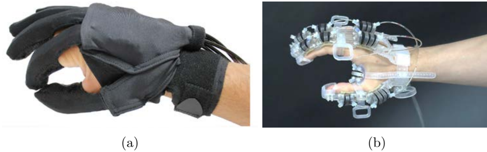
Figure 1.2: Soft pressurizable hand exoskeletons: (a) Polygerinos et al. [20] and (b) SNU Exo-Glove PM [23] (reproduced with the permission of the authors).
