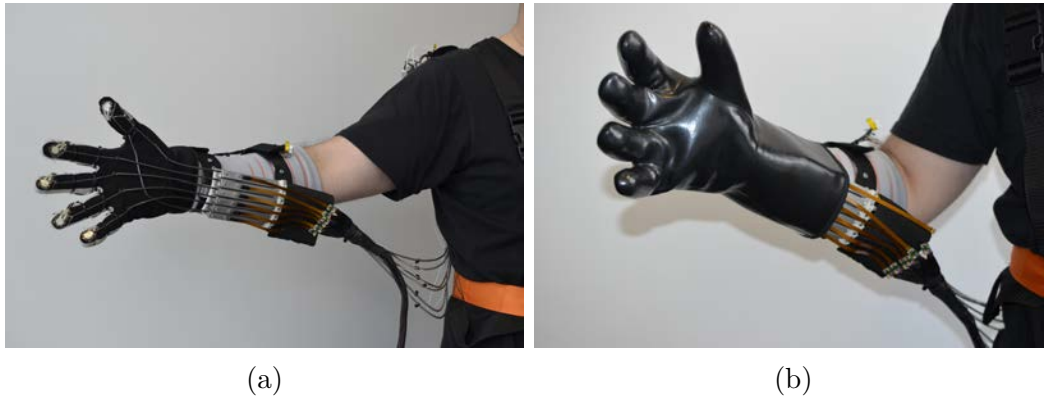
Figure 6.3: HEMS glove: (a) internal glove with the tendon and actuation systems and (b) external glove.
