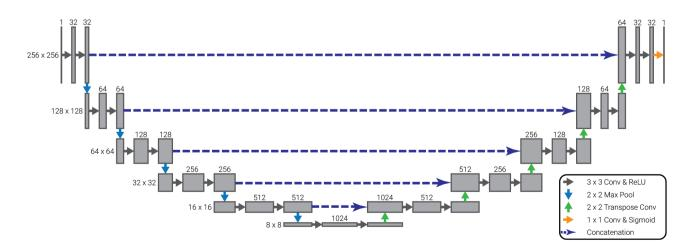
FIGURE 1 An overview of the network architecture
