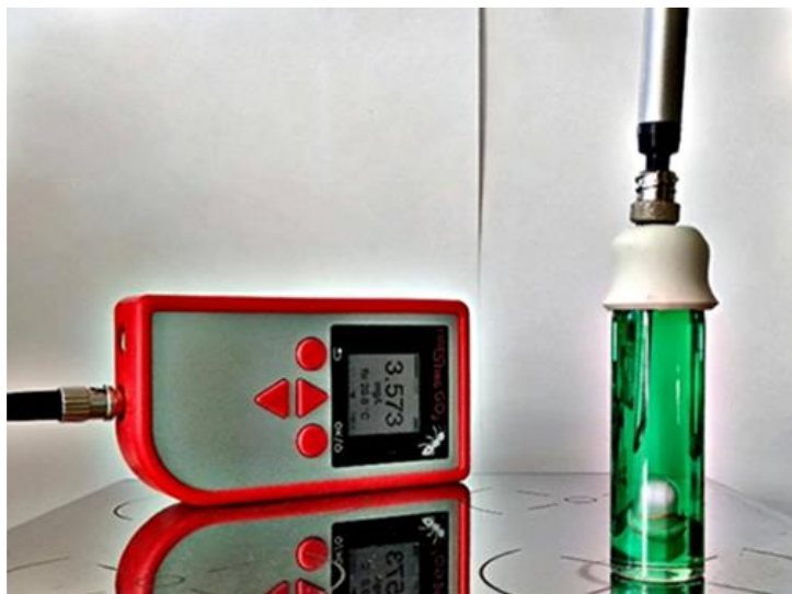
Figure 2-7. Setup of the in-situ monitoring of the dissolved O 2 concentration in a typical, not externally deoxygenated, Cu(0)-mediated RDRP.
