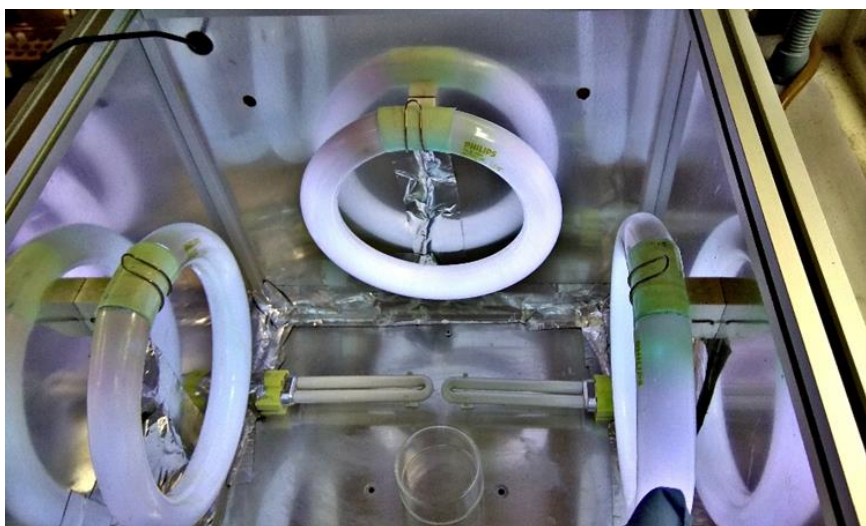
Figure 3-33. Custom-made UV box setup for the high-scale polymerizations with 4 9-W bulbs, broad band emission and \lambda_{\text{max}} \sim 360 nm.
