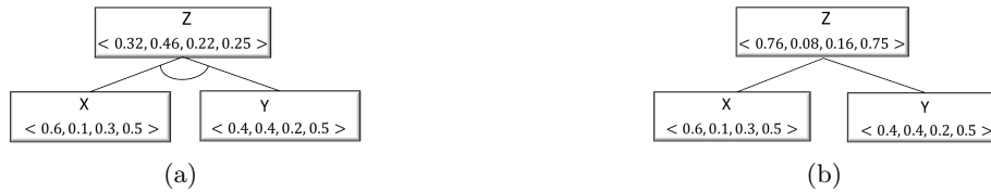
Fig. 2: Computing an opinion on event Z via (a) AND gate, and (b) OR gate.
