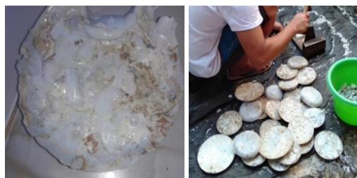
Figure 3. Melted PET plastic waste after extraction from moulds
