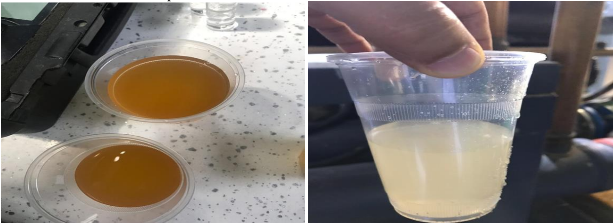
Figure 9 (a): Water of the circle before adding the inhibitor, (b): Water of the circle after adding the inhibitor
