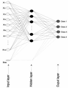
Fig. 3. Multilayer perceptron with one hidden layer.
