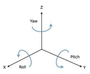
rotations around their specific axis. The sensing of angular velocity makes the gyroscope beneficial for measuring motion in several devices.
