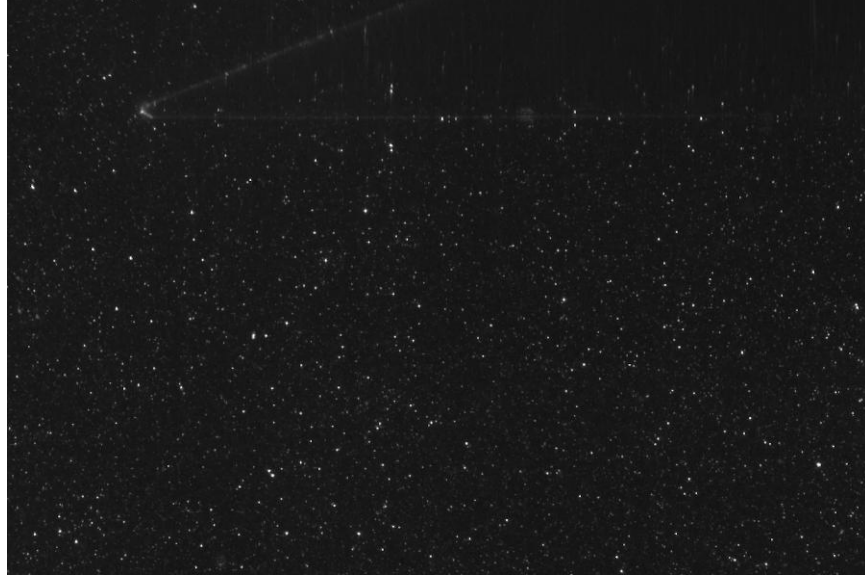
Figure 4.7: Cropped sample PIV image from flat plate experiments
