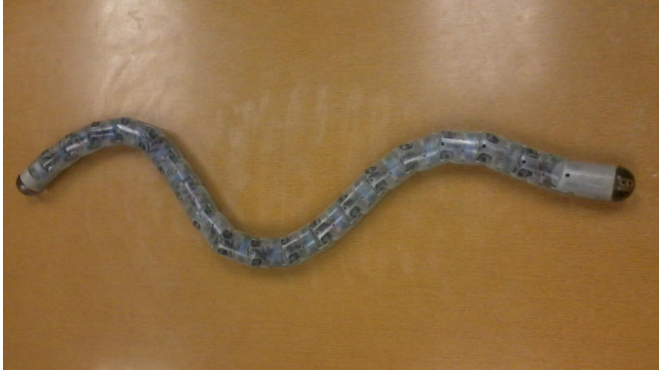
Figure 6.2: NEELBOT-1.1 on a tabletop without its waterproofing skin (from (Potts, 2015))
