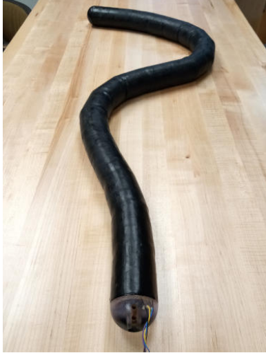
Figure 1.1: Photograph of NEELBOT with its black latex waterproofing skin
